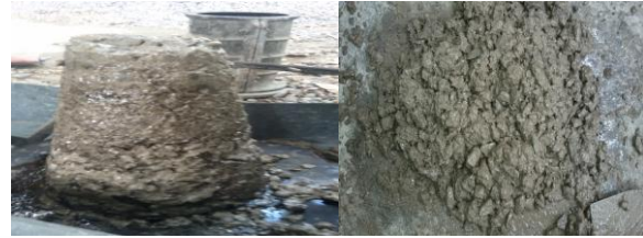
Fig 1: Slump cone test of Geopolymer Concrete
